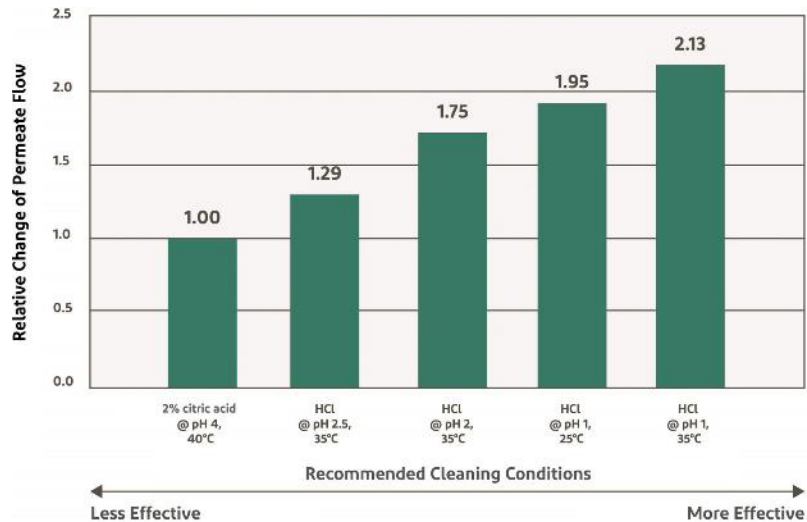
Figure 49: Effect of pH on the removal of calcium carbonate
