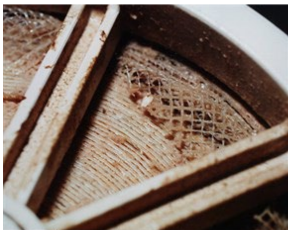
Figure 61: High pressure drop due to biofouling has pushed out the feed spacer
