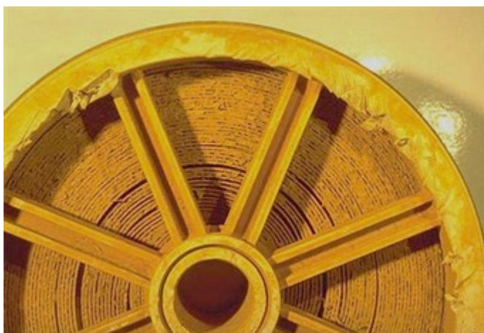
Figure 56: Picture of iron fouled feed side of an element with telescoping damage and signs of mechanical force
