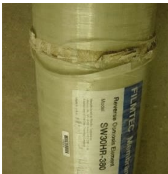
Figure 60: Picture of damaged fiberglass shell
