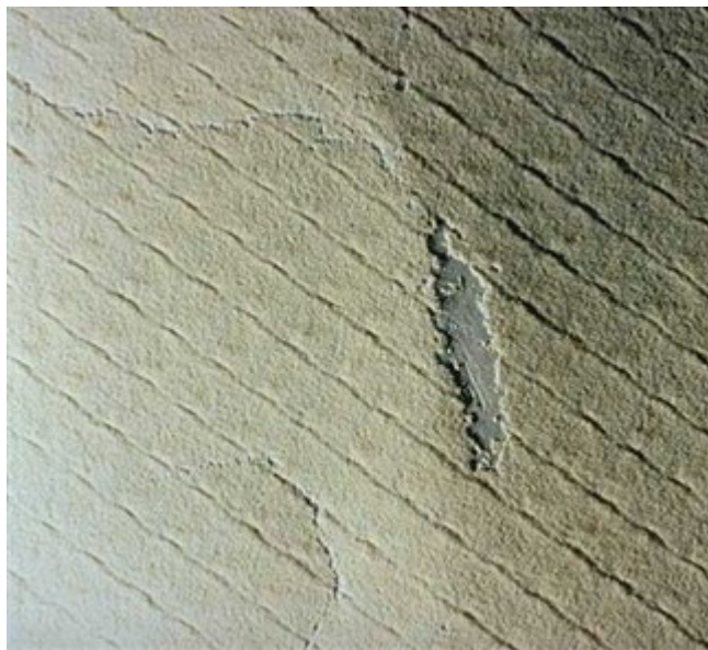
Figure 57: Picture of scaled membrane surface with imprints from the feed spacer
